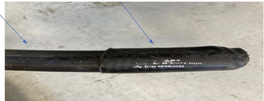
Heat shrink seal to prevent conductor corrosion during storage and installation
